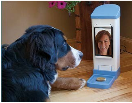
Figure 3: ICPooch an interactive two way video and food dispensing device for dogs and cats. [17]
